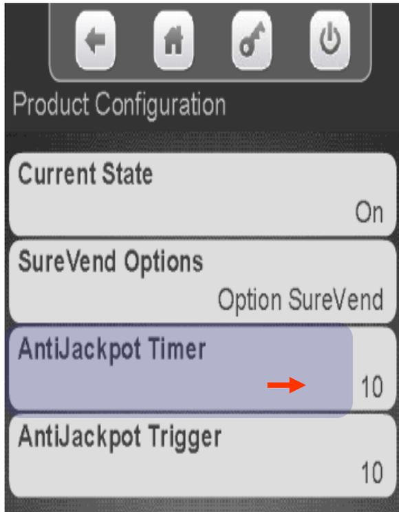
Use the Keypad to enter a new time (in minutes) and press Done. If a spiral turns 3 times and no product is detected by the SureVend™ sensor, that selection will be unavailable for the period of time set. After the AJT is expired, the selection will be available for purchase again, The SureVend™ will protect the customer from losing money during this time.
